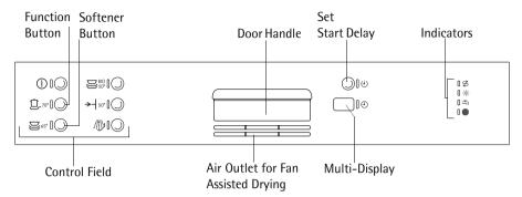
The **Control Field** comprises the ON/OFF switch (1) and the programme buttons with LED indicators.
